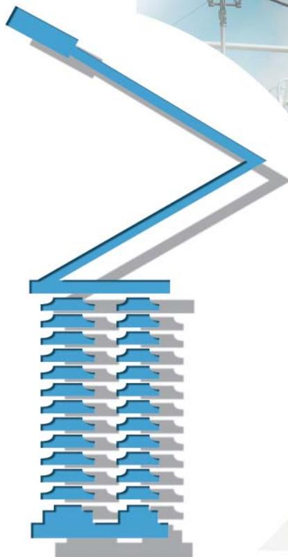
In service since 1954 (3000 3-pole installed since then), the Pantograph System Disconnecter (SSP) is a device for vertical disconnection that separates 2 stacked horizontal layers.
