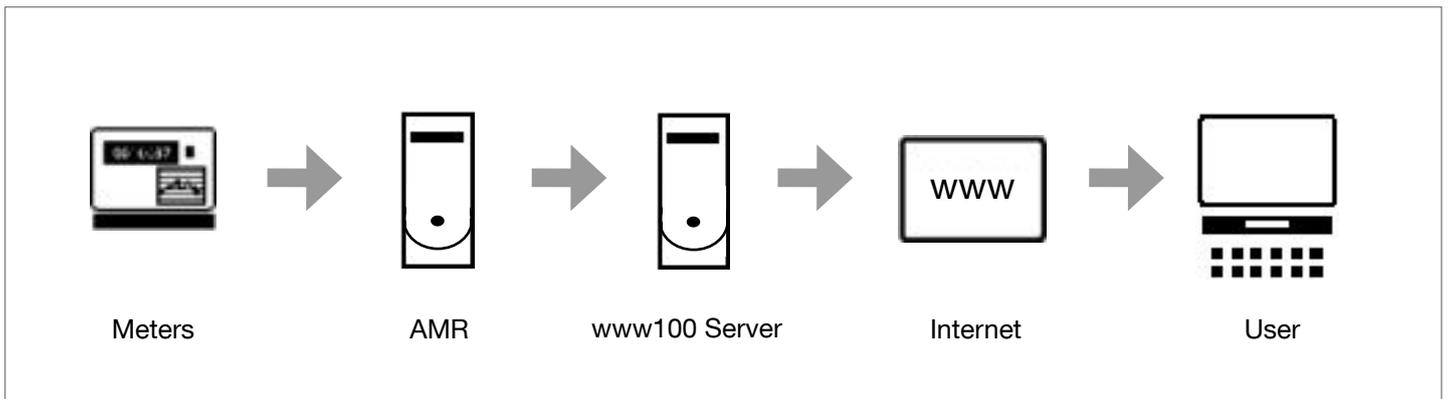
The main purpose of www100 is distribution of metering data via network.
