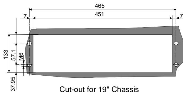
Cut-out for panel-flush mounting
