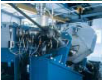
Extruding and centring. Latest technology extrusion head and eccentricity-measuring instrument for catenary line.
