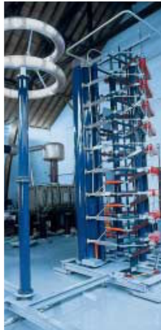
Lightning impulse testing. Impulse generator in the high-voltage laboratory for lightning and switching impulse testing of high-voltage cables and accessories (impulse voltages up to 1.8 MV).
