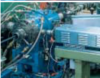
Horizontal curing. Horizontal triple-head extrusion machine, type MDCV, with long-land die for dry curing.
