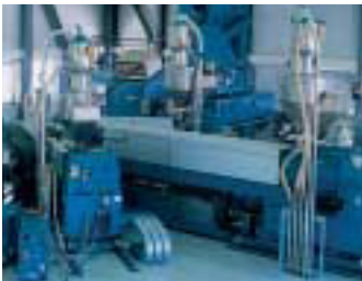
Superextruder. High-performance extrusion plant, type CDCC, with materials feed under controlled "clean room" conditions.
