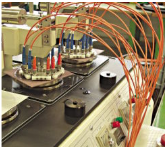
LWL-Steckverbinder/Poliervorgang Fiber optic connectors/Polishing procedure
