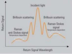
DTS utilizes the Raman effect to measure temperature. An optical laser pulse propagating through the fiber gets scattered light back to the transmitting end, where it is analyzed. The intensity of the Raman scattering is a measure for the temperature along the fiber. The position of the temperature reading is determined by measuring the arrival timing of the returning light pulse similar to a radar echo.
